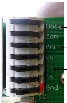
From DCSAP "Wnc" to WATCHMAN TB2 "S2" Green Wire (Wnc=Warning normally closed contact)
